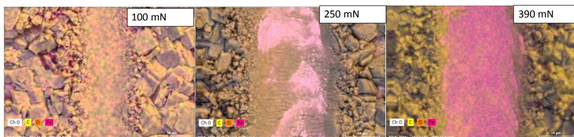
Figure 14. EDS mapping analysis of constant load scratch tests at different forces.
